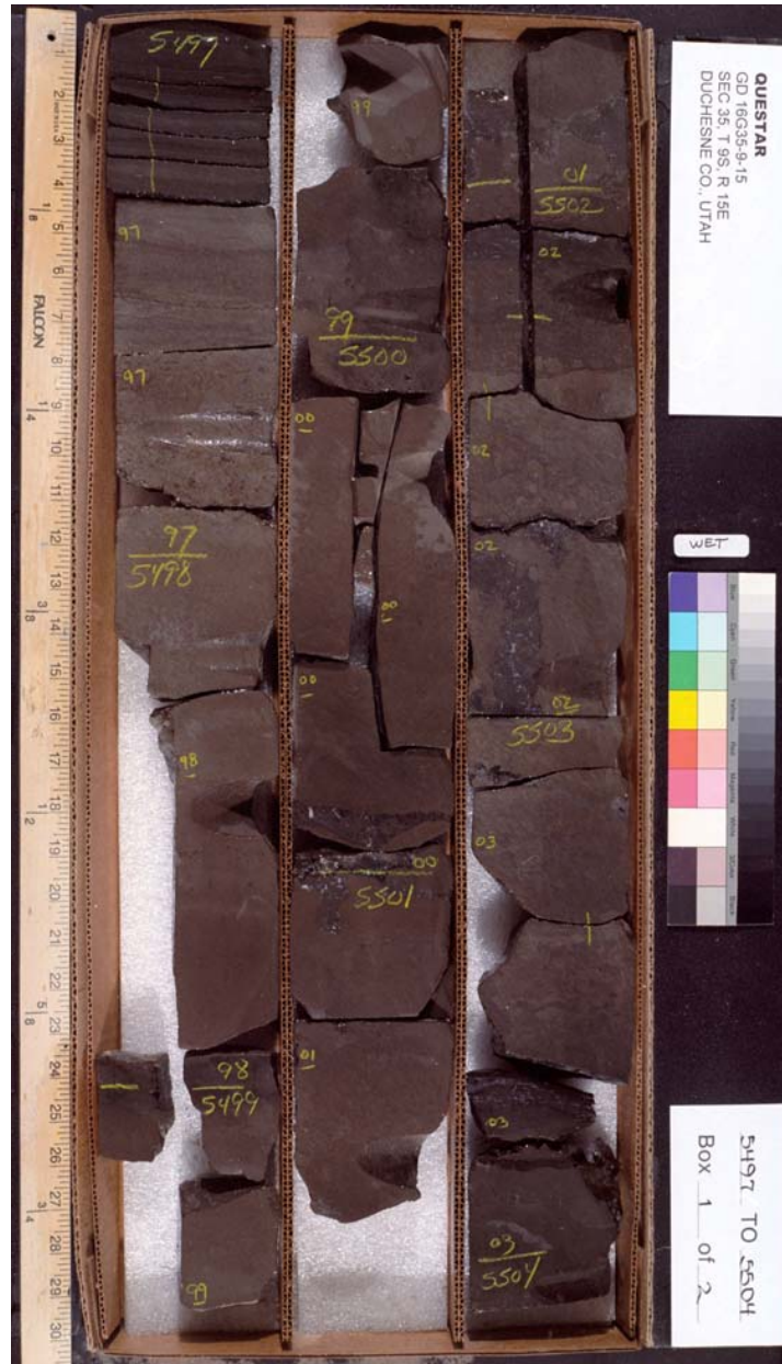
Figure 4. Core from the Uteland Butte Member of the Green River Formation, Uinta Basin, Utah (QEP Resources, GD-1G-35). The lighter tan interval shown in this box is equivalent to the productive zone in the Bill Barrett (figure 2) and Berry/Lynn (figure 3) cores, but is thicker in this area (~8 feet thick).
