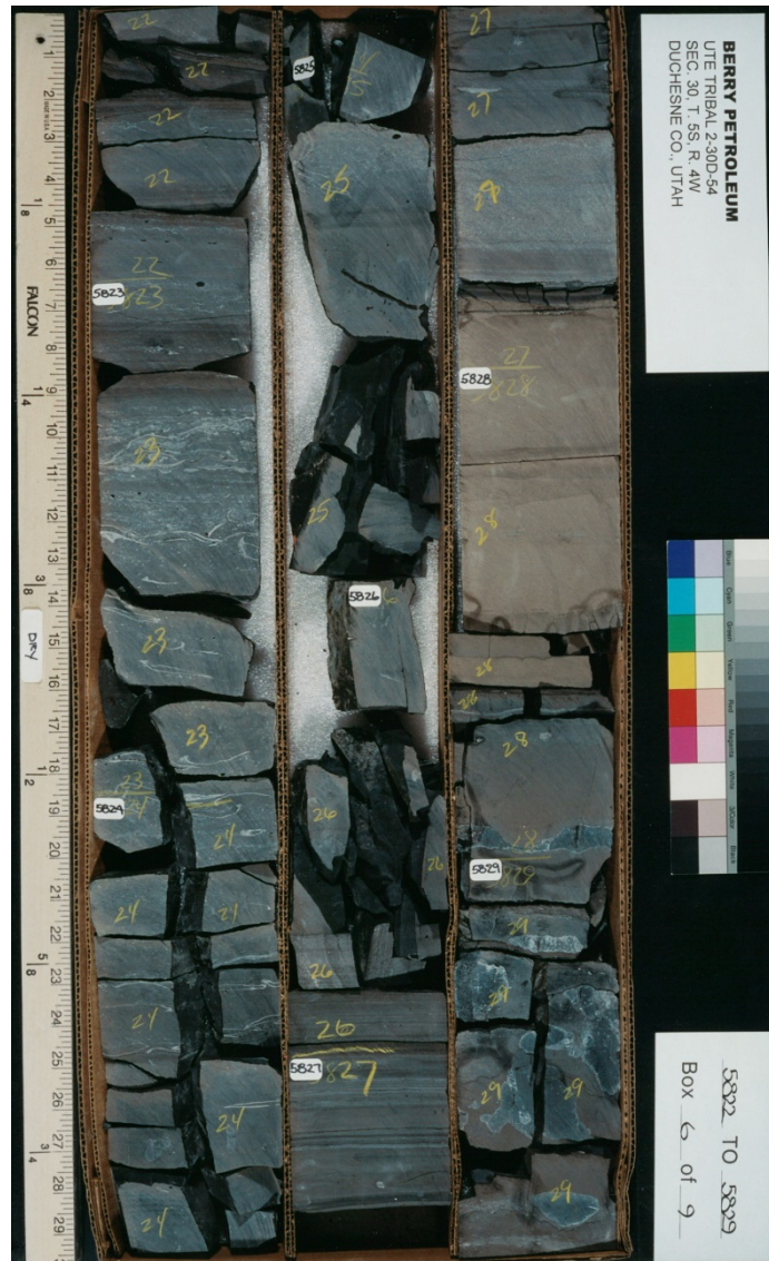
Figure 3. Core from the Uteland Butte Member of the Green River Formation, Uinta Basin, Utah (Berry/Lynn Energy, 2-30D-54). The lighter tan interval at right is equivalent to the productive zone in the Bill Barrett core (figure 2), but is much thinner in this area (~2 feet thick).
