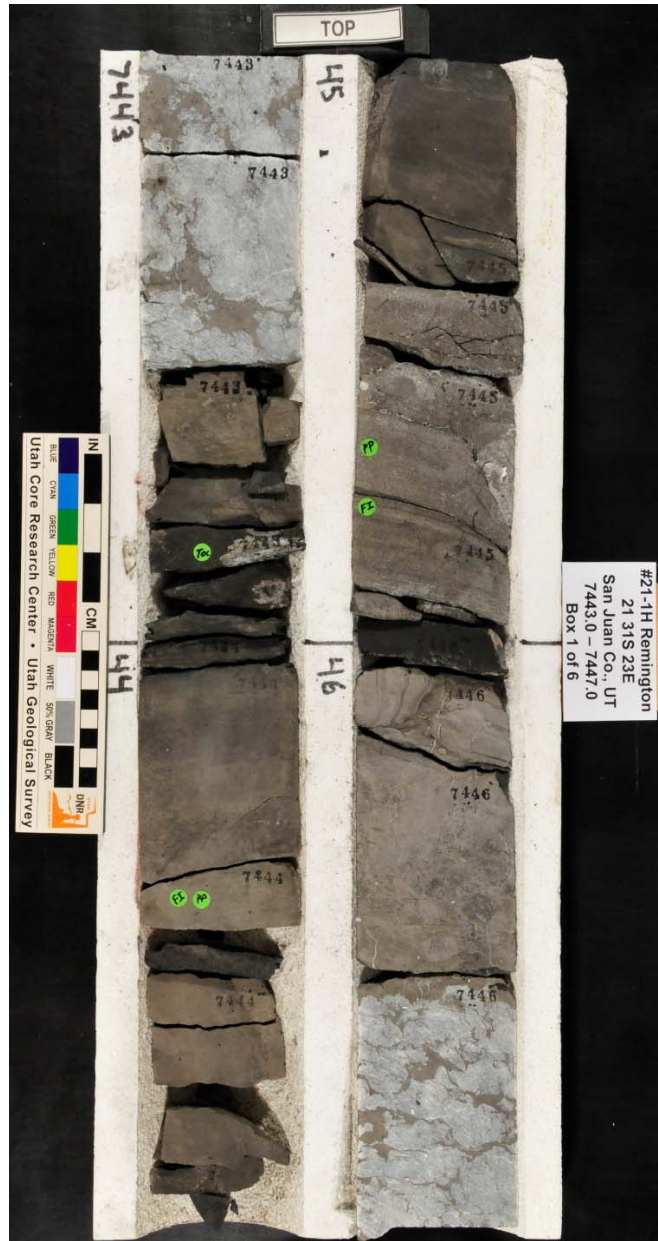
Figure 6. Core from the Cane Creek shale of the Paradox Formation, Paradox Basin, Utah (Union Pacific Resources Company, Remington 21-1H). The source of the oil is the dark gray to black, organic-rich shale intervals, which are interbedded with mottled anhydrite (lightest gray).
