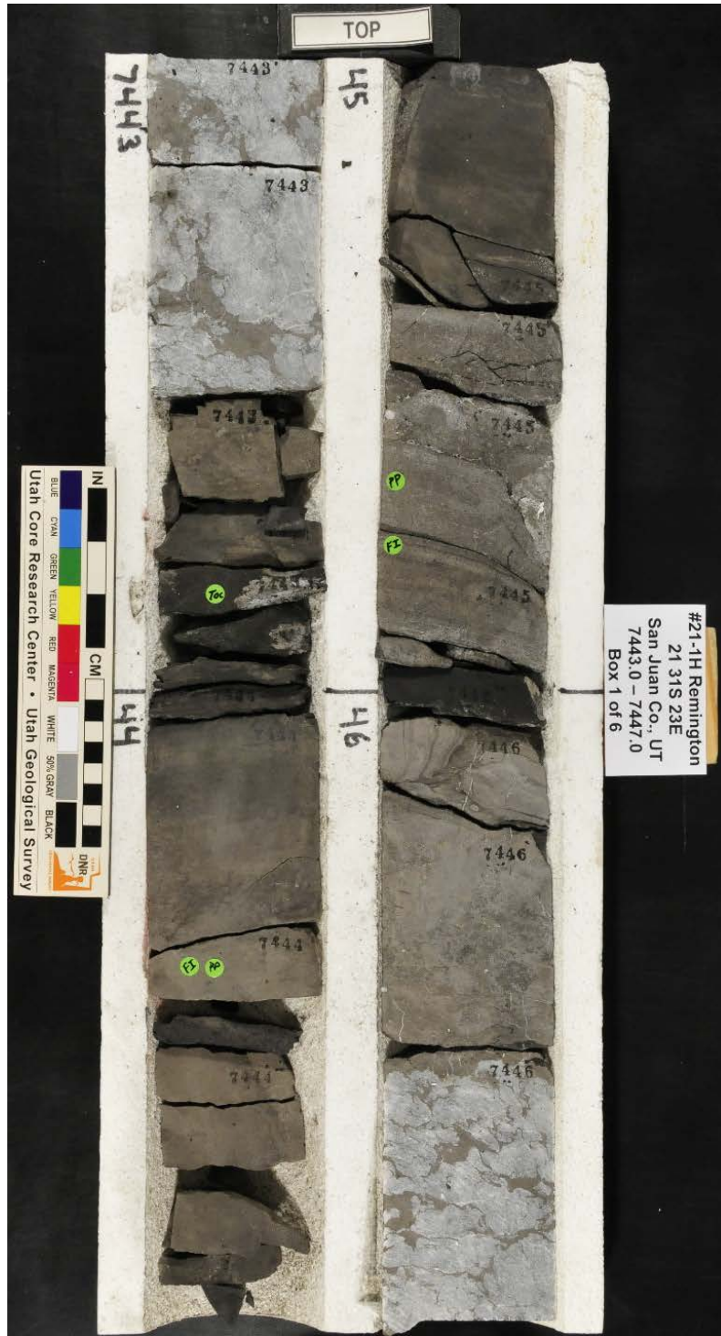
Figure 8. Cane Creek shale zone core from the Union Pacific Resources Remington 21-1H well (section 21, T. 31 S., 23 E., SLBL&M, San Juan County, Utah) displays interbedded medium gray dolomite with organic-rich dark gray/black shale. Also present is mottled light gray to white anhydrite.
