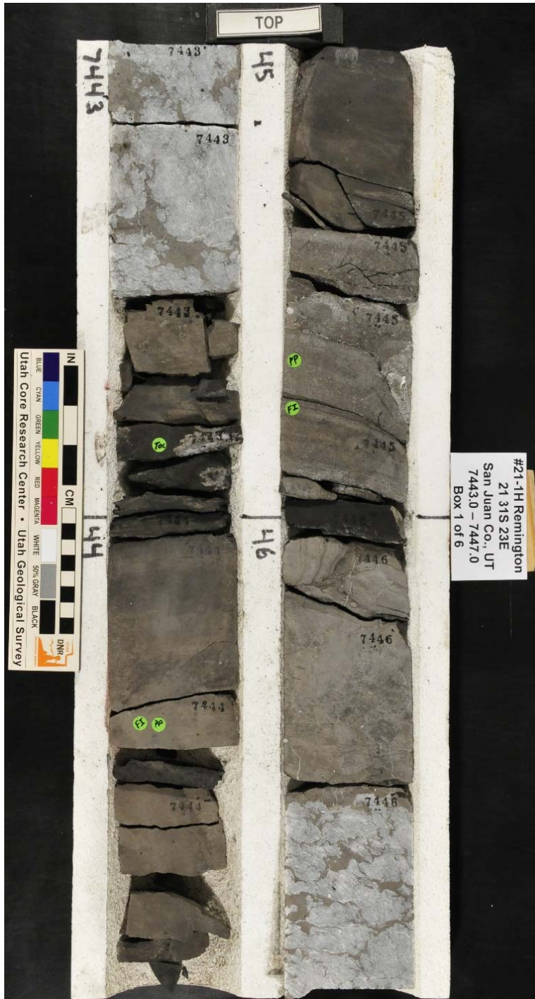
Figure 8. Cane Creek core from the Union Pacific Resources Remington 21-1H well (section 21, T. 31 S., 23 E., SLBL&M, San Juan County, Utah) displays interbedded medium gray dolomite with organic-rich dark gray/black shale. Also present is mottled light gray to white anhydrite.
