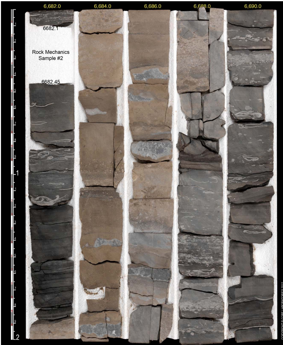
Figure 2. Uteland Butte core from the Bill Barrett 14-1-46 well. The horizontal drilling target is the roughly 5-ft light brown dolomitic interval. Porosity in this interval ranges from 15-30% and permeability averages 0.06 mD. The dolomite is interbedded with organic-rich mudstones and limestones averaging between 1% and 3% TOC. Note the abundant shell fragments indicating deposition in a freshwater lacustrine environment.
