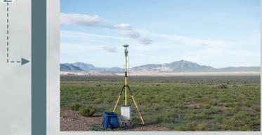
**ABOVE:** Gravity survey equipment (CG-5 gravimeter and GPS tripod) with Iron Mountain in the background
