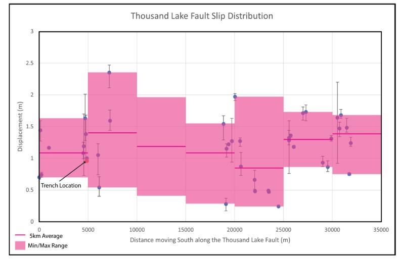
**Figure 3.** Mean, minimum, and maximum displacement values for each profile were obtained using the Scarp\_VS program. Values were averaged within each 5km stretch of the TLF in order to calculate cumulative Moment for the MRE (**figure 4**).
