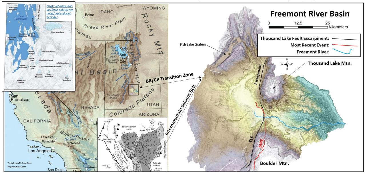
**Figure 1.** The TLF represents one of the easternmost Basin and Range faults within Utah. The TLF separates a province of units deformed by Sevier-Laramide orogenic activity and subsequent extension from the relatively undeformed laterally continuous units of the Colorado Plateau.
