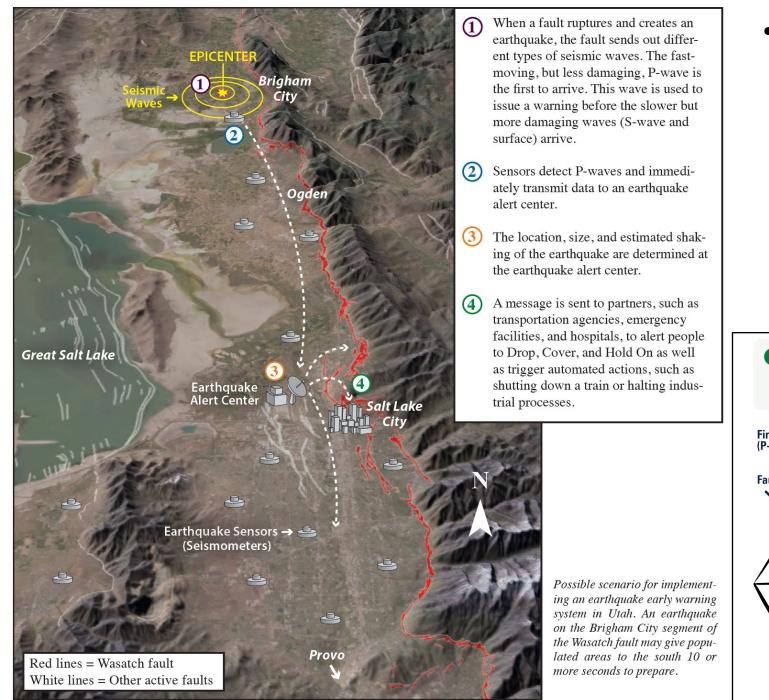
Scenario for a hypothetical EEW system activation for an earthquake on the Brigham City Segment of the Wasatch Fault Zone
