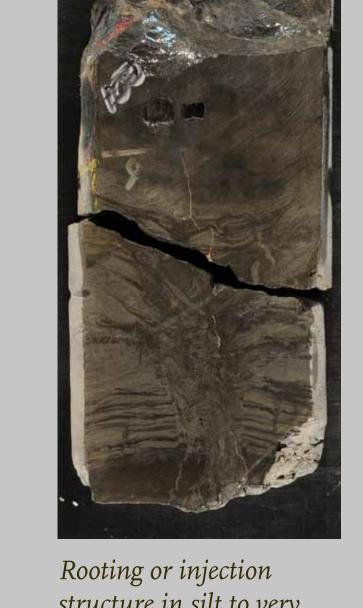
Rooting or injection structure in silt to very
