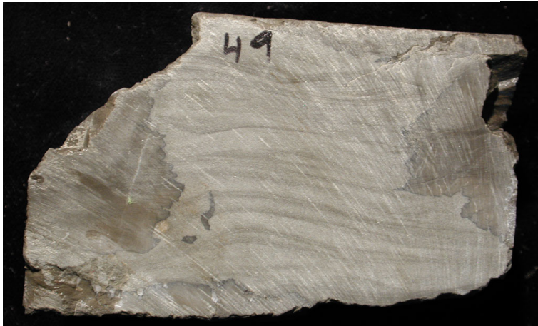
Figure 4. Typical Twin Creek Limestone, Watton Canyon Member, from the UPRR No. 3-3 well (section 3, T. 2 N., R. 7 E., SLBL, slabbed core from 8749 feet) showing finely laminated, carbonate mudstone deposited in backbank, low-energy brackish water environment. Note that essentially no porosity is present.
