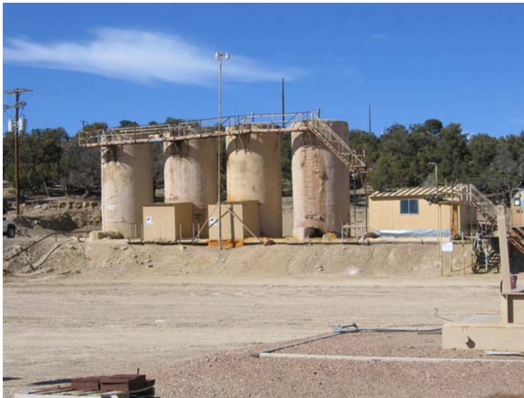
Figure 5. Insulated tanks and heat treater at the Ute Fee 2-33C6 well in Cedar Rim field, SW1/4SW1/4 section 33, T. 3 S., R. 6 W., UBLM.
