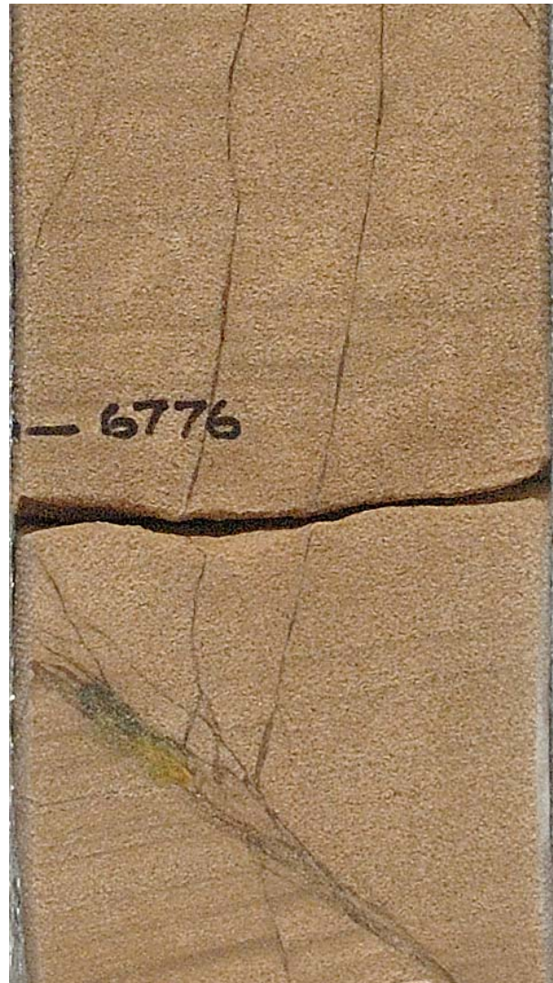
Figure 14. Early, bitumen and gouge-filled, silica-cemented, impermeable fractures, with slight offsets, in the Navajo Sandstone, from the Kings Meadow Ranches No. 17-3 well (slabbed core from 6776 feet), Covenant field.
