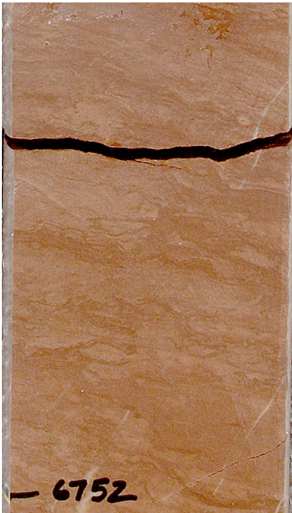
Figure 13. Typical middle unit of the Navajo Sandstone, from the Kings Meadow Ranches No. 17-3 well (slabbed core from 6752 feet), Covenant field, showing siltstone laminae and shale deposited in an interdune environment.
