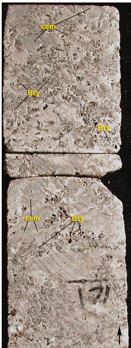
Figure 26. Typical Ismay-zone bryozoan-mound lithofacies showing large tubular bryozoans (Bry) and “lumps” of marine cement (cem). Scattered phylloid-algal plates are also present. This mound fabric is typical of higher energy, and possibly shallower water than the mud-dominated fabrics. Mustang No. 3 well (section 26, T. 36 S., R. 25 E., SLBL&M), Mustang Flat field, San Juan County, Utah, slabbed core from 6171 feet.
