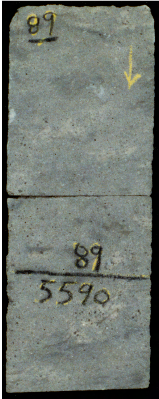
Figure 29. Typical Desert Creek-zone dolomitized grainstone, calcarenite lithofacies; North Heron No. 35-C well (section 35, T. 41 S., R. 25 E., SLBL&M), Heron field, San Juan County, Utah, slabbed core from 5589 feet.
