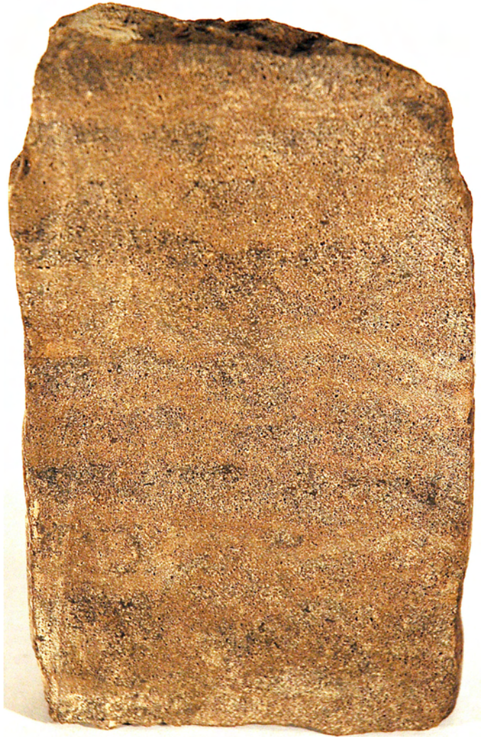
Figure 30. Typical Desert Creek-zone oolitic grainstone; Aneth No. 27-D-4 well (section 27, T. 40 S., R. 24 E., SLBL&M), Greater Aneth field, San Juan County, Utah, slabbed core from 5620 feet. Note excellent moldic porosity development.
