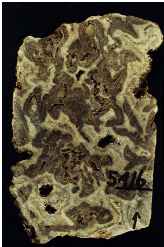
Figure 42. Typical pattern of marine cementation within the well-lithified Desert Creek zone “wall” complex. Figure 3-20. Slabbed core segments from the Blue Hogan No. 1-J-1 well Blue Hogan No. 1-J-1 well (section 1, T. 42 S., R. 23 E., SLBL&M), slabbed core from 5415.5 to 5416.1 feet, Desert Creek field, San Juan County, Utah.
