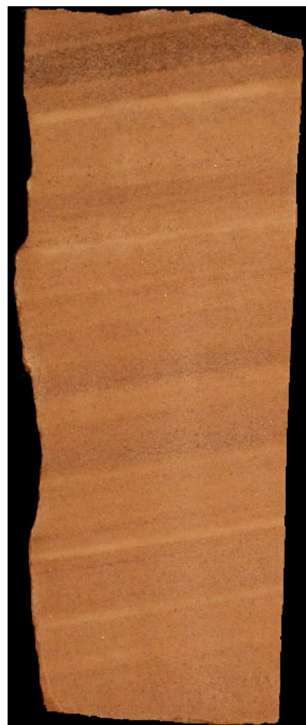
Figure 7. Typical Nugget Sandstone, from the Champlin No. 1 McDonald 31-3 well (NWNE section 3, T. 2 N., R. 7 E., SLBL, slabbled core from 9872 feet), Pineview field (figure 2), showing cross-bedding in fine-grained sandstone deposited in a dune environment.
