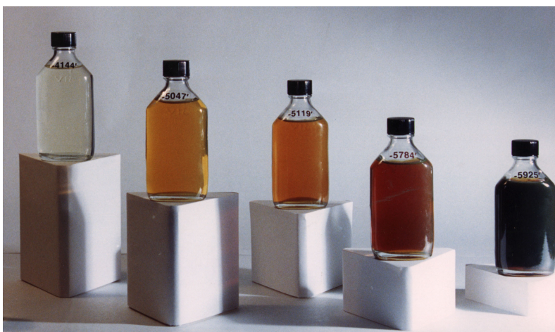
Figure 23. Color changes in retrograde condensate from Anschutz Ranch East field, Summit County, Utah. Sample bottles are labeled with subsea structural elevation.
