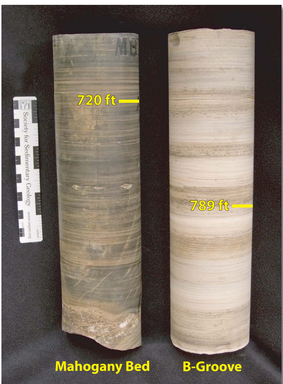
Core from the P-4 well illustrating the color difference between the rich Mahogany Zone and lean B-Groove.
