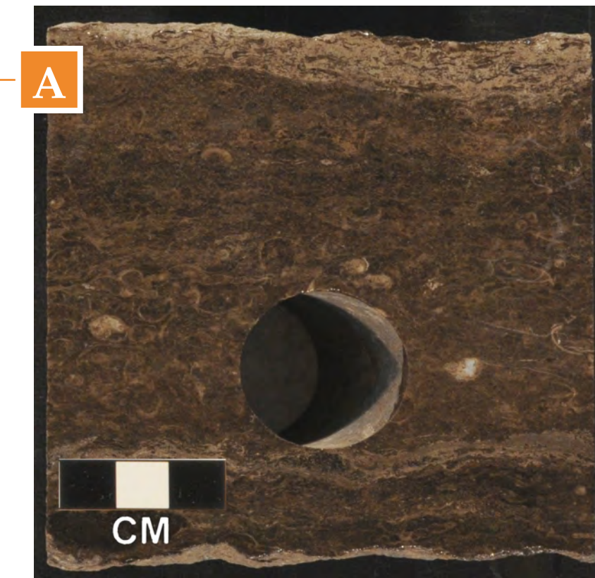
A - Conventional core segment showing vaguely laminated MISS (Microbially Induced Sedimentary Structures). Federal No. 15-24B core (West Willow Creek field), 4786.5 ft.
