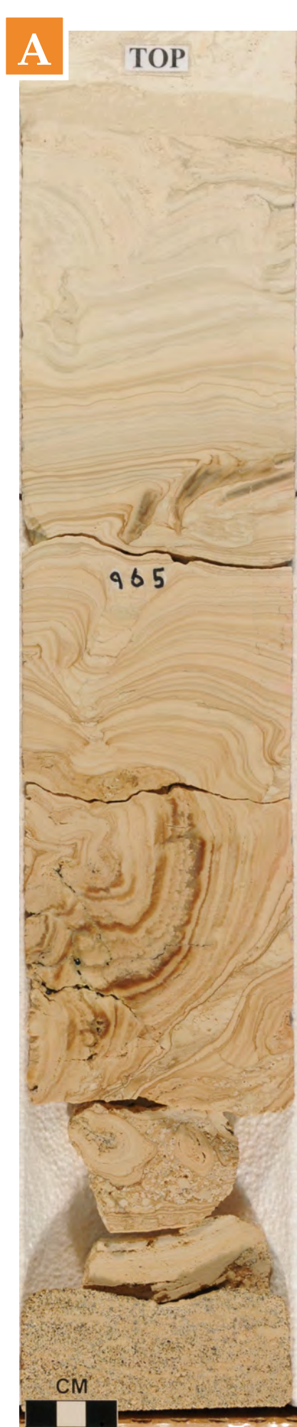
A - Large stromatolite domal head in which the synoptic relief diminishes upwards. Oolitic/peloidal sediments fill the space between stromatolites. The stromatolite grew on an oolitic/pisolitic/ oncolitic substrate. Skyline 16 core, 964.5-966.0 ft.
