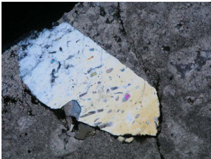
Figure 42. Relatively large quartz crystal from the Lisbon No. D-616 well at 8356 feet. Small oriented grains of anhydrite are encapsulated in the quartz. Width of image is 1.3 mm.
