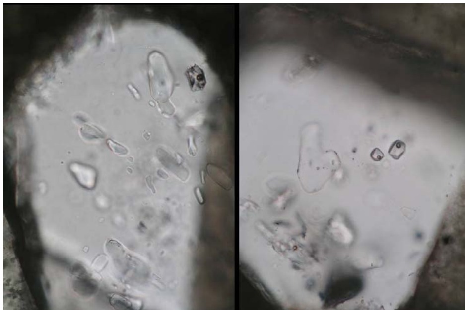
Figure 44. Primary liquid-rich inclusions in quartz from the Lisbon No. D-616 well at 8356 feet. Height of image is 0.3 mm. Irregularly shaped inclusions are anhydrite.
