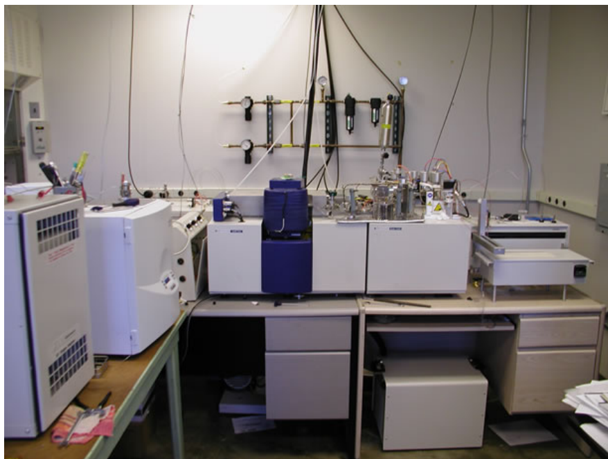
Figure 56. The CSM Stable Isotope Laboratory's GV Instruments IsoPrime stable isotope ratio mass spectrometer. Several peripheral devices are interfaced with the IsoPrime for both dual-inlet and continuous flow applications.
