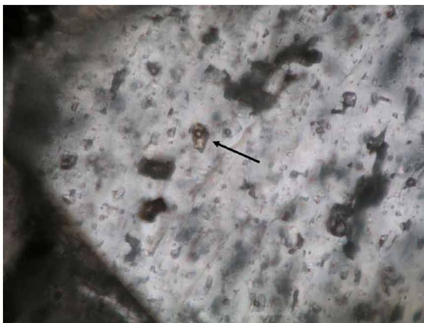
Figure 32. Brown primary oil inclusion (arrow) in calcite from the Lisbon No. D-616 well at 8356 feet. Clear inclusions are aqueous. Width of image is 0.3 mm.
