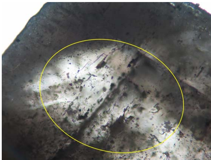
Figure 38. Low-magnification image of saddle dolomite shown in figure 35. Dark growth zones are truncated near the left side of the oval. Oil inclusions in figure 35 occur in the light colored dolomite on right side of oval. Width of image is 0.7 mm.
