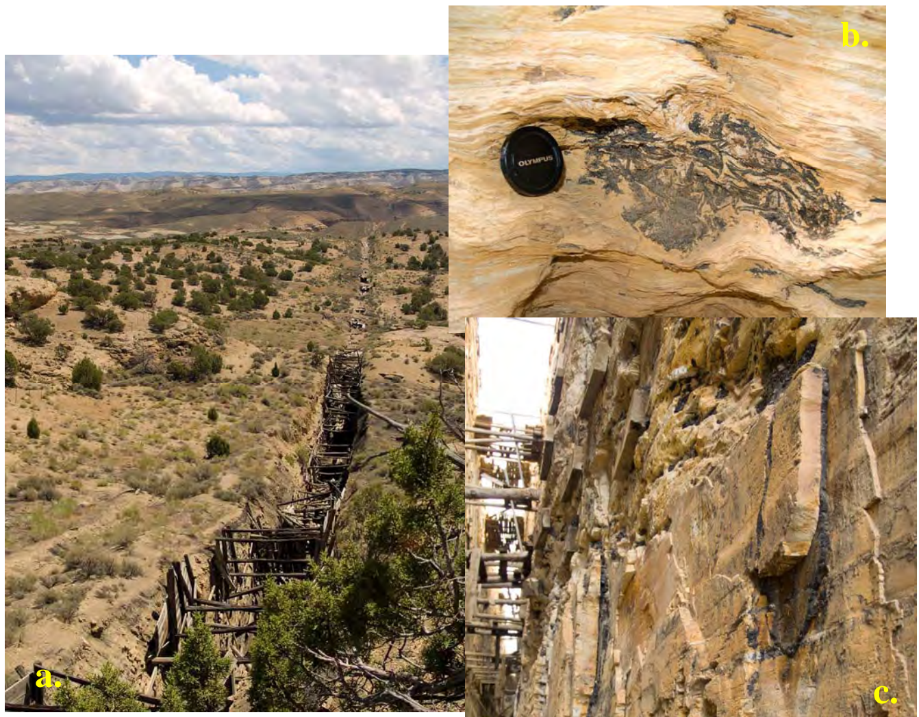
Figure 7. a. Mined-out Cowboy gilsonite vein. b. Gilsonite within a dissolved saline mineral cavity; notice the blade-like shape of the replaced nahcolite crystals. c. Gilsonite in vertical fracture.
