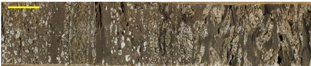
Figure 3. Core from the South Uinta Basin 12 well. Notice the smaller, partially-dissolved nahcolite crystals (yellow bar equals one inch).
