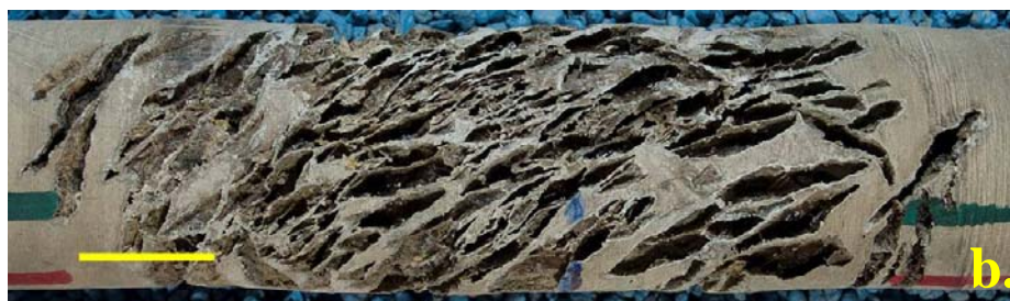
Figure 2. a. Nahcolite nodules within the Utah State 1 core displaying no dissolution (depth – 1825.6 ft) (yellow bar equals one inch). b. Dissolution of nahcolite in the Utah State 42-34 core (depth – 1795.0 ft).
