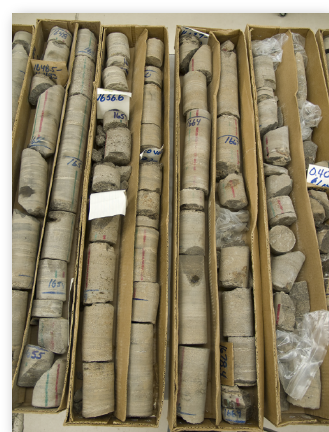
Well 42-33 (1648-1671 ft) - Dissolution of saline minerals; each white tag represents a 0.5 to 1.5 ft void left behind by a dissolved nahcolite nodule.
