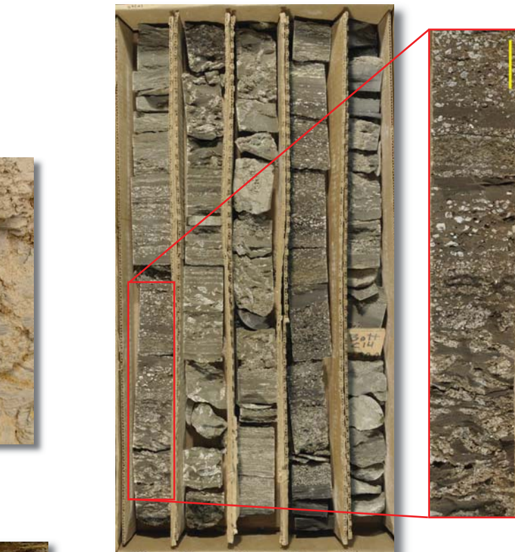
Photo 1 - 221-231 ft Nahcolite/shortite crystals - partially dissolved
