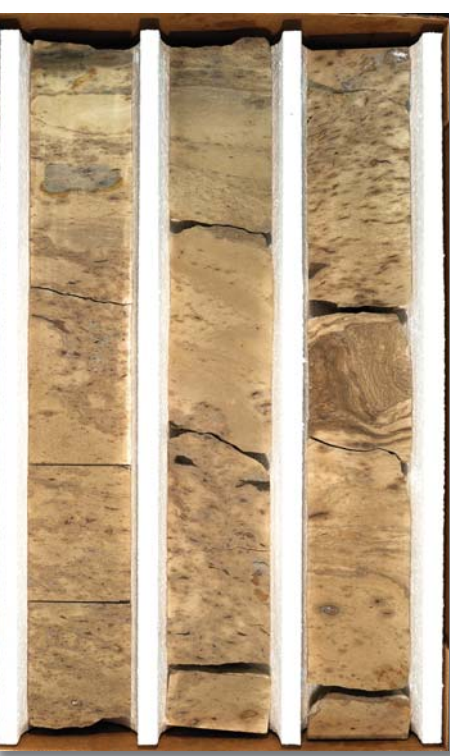
Photo 1 - 300-306 ft Highly porous volcaniclastic debris flow with mud rip-up clasts
