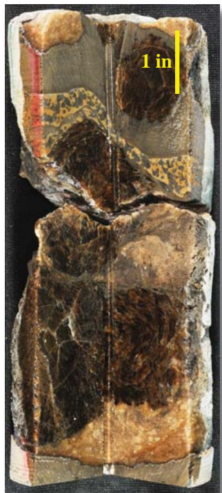
Intact nahcolite nodule in the Utah State 1 core (1825 ft).
