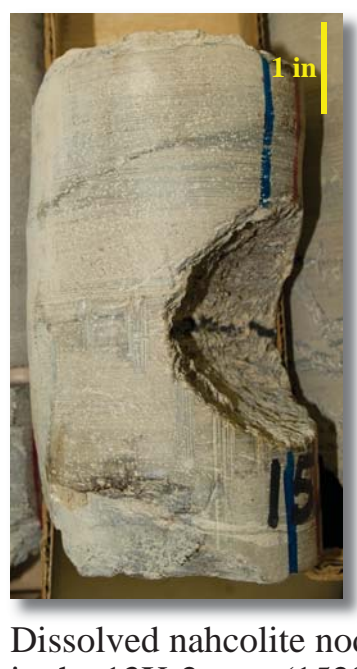
Dissolved nahcolite nodule in the 13X-2 core (1528 ft).
