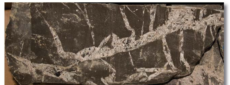
Intact saline mineral fracture fill in the 13X-2 core (1580 ft).
