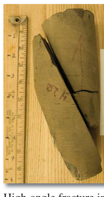
High-angle fracture in the P-1 core (420 ft).
