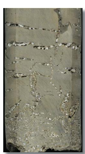
Dissolved saline mineral fracture fill in the P-4 core (365 ft).
