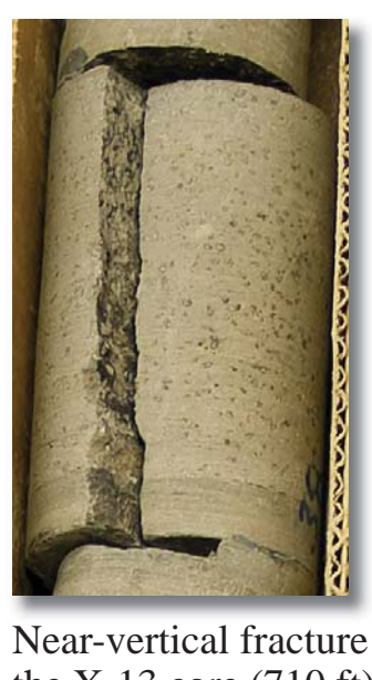
Near-vertical fracture in the X-13 core (710 ft).
