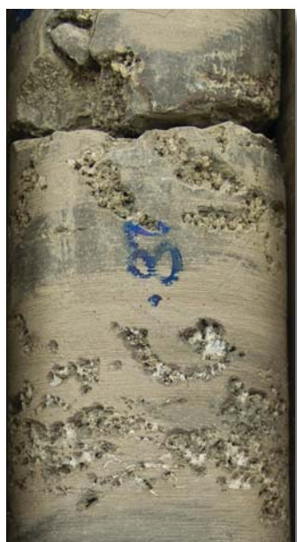
Dissolved saline mineral fracture fill in the X-13 core (671 ft).
