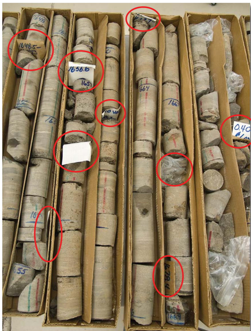
The Birds Nest aquifer in the 42-34 core (1648-1671 ft). The slips of paper (red circles) represent 0.5-1.0 foot gaps in the core created from the dissolution of nahcolite nodules.
