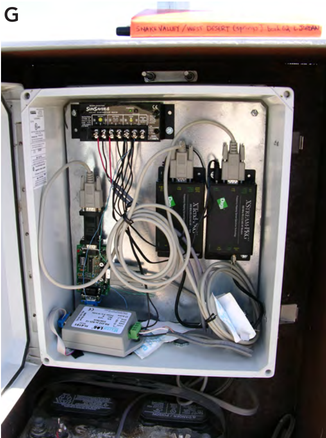
Figure 5.6. continued G. Weatherproof box housing radios, solar panel power controller, and data card inside protective metal box.
