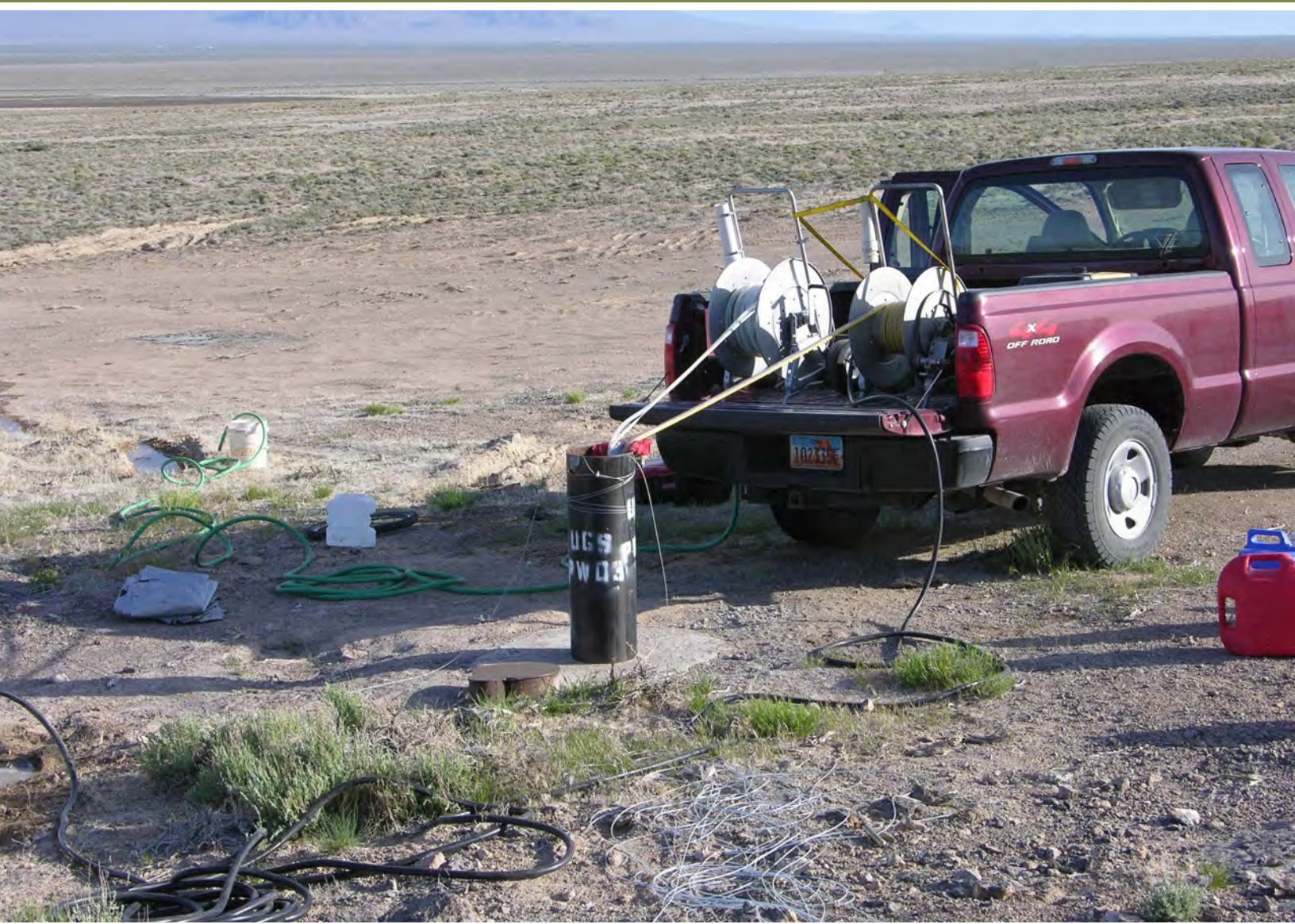
Pumping piezometers PW03A and PW03B at site 3 for hydrochemical sampling.
