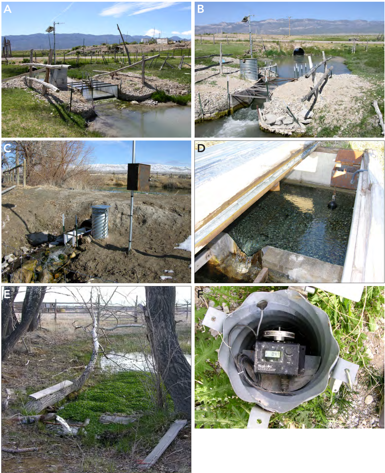
Figure 5.6. Instrumentation at surface-flow measurement sites. A. 20 cfs ramp flume at West Middle Ditch (site 28) and large stilling well, solar panel, and antenna to left of flume. B. 3-foot Parshall flume at East Middle Ditch (site 28). C. 8-inch Palmer Bowlus flume to left of stilling well and instrument box on pole downgradient of the earthen dam at Miller Spring (site 32). D. 90-degree v-notch weir plate (lower left) and float on pulley (upper right) attached to a shaft encoder (concealed in metal box) at Clay Spring (site 29). E. Ultrasonic flow meter transducers attached to discharge pipe at Kell Spring (site 31). F. Shaft encoder and pulley system inside a stilling well.
