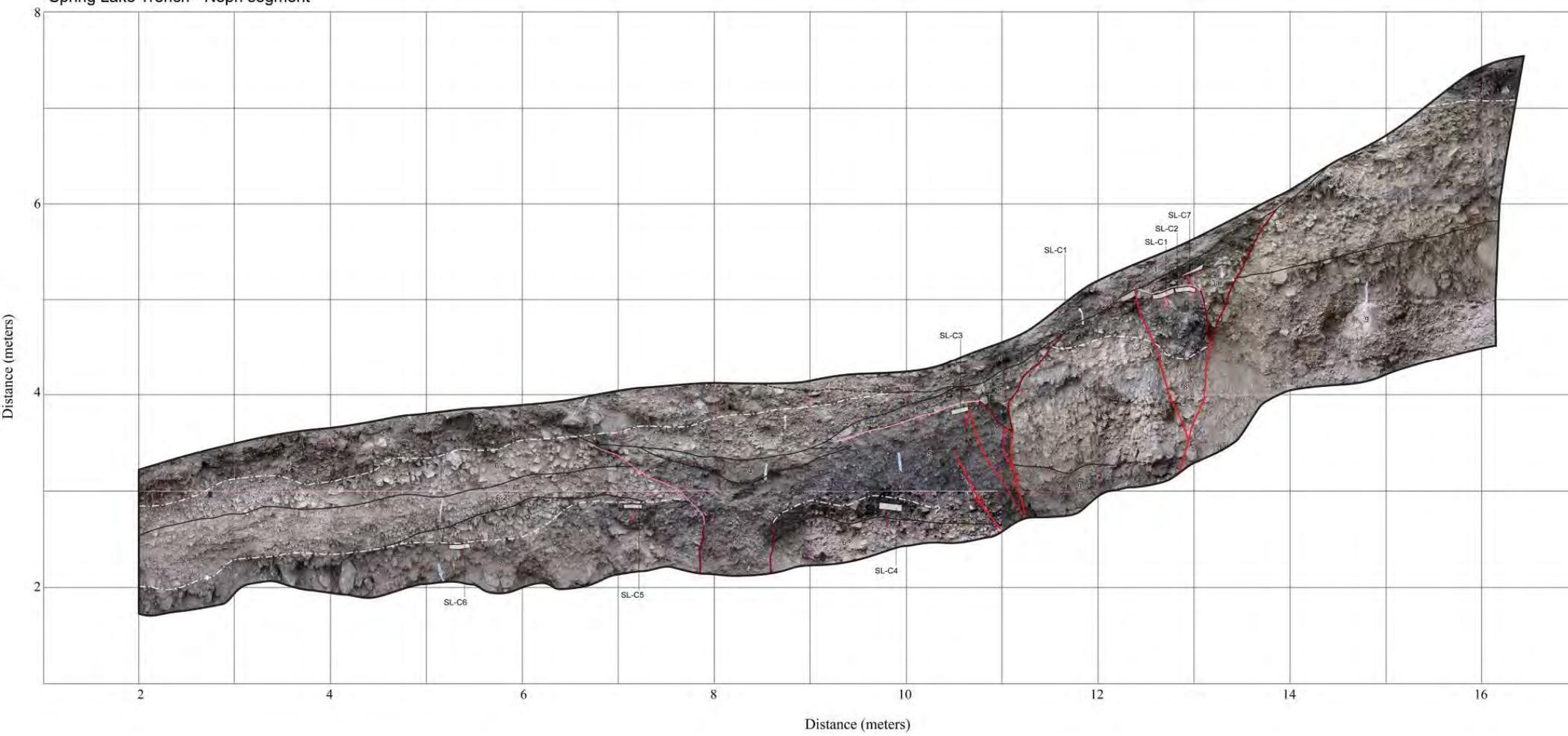
Photomosaic of the north wall (by Chris DuRoss) with interpretations of faults and sedimentary units.
