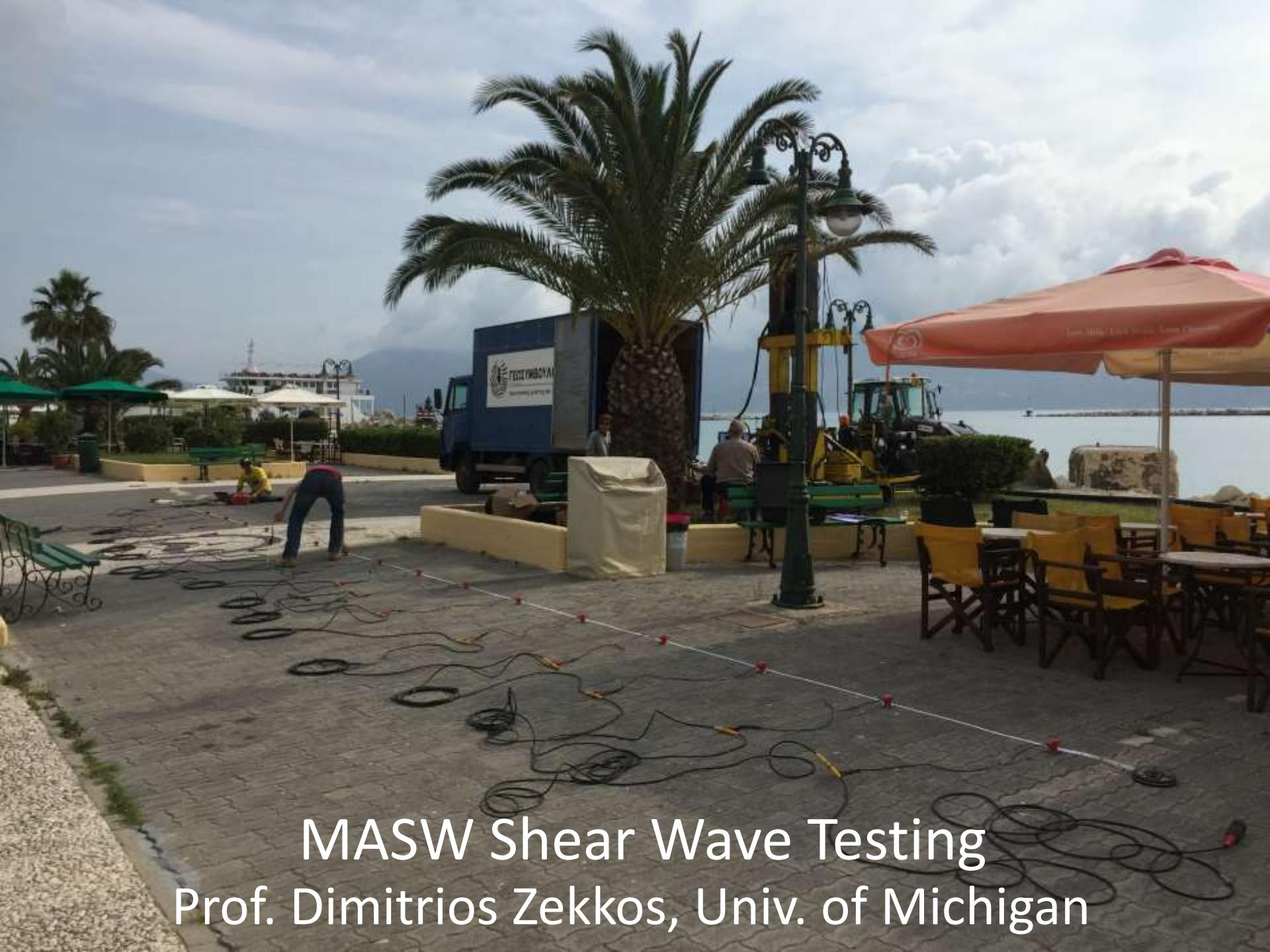
MASW Shear Wave Testing
