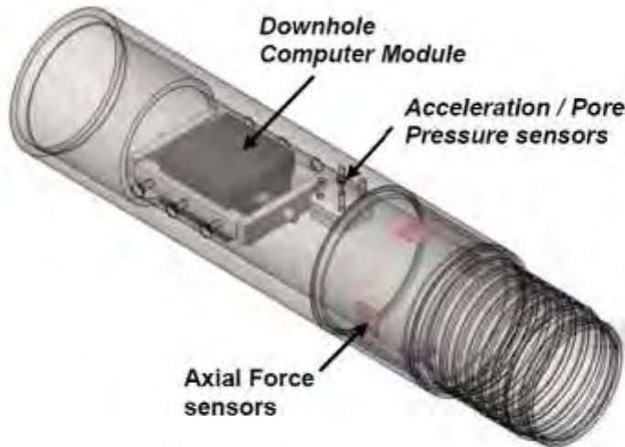
FIG. 1. iBPT testing equipment (after Thurairajah 2013).
