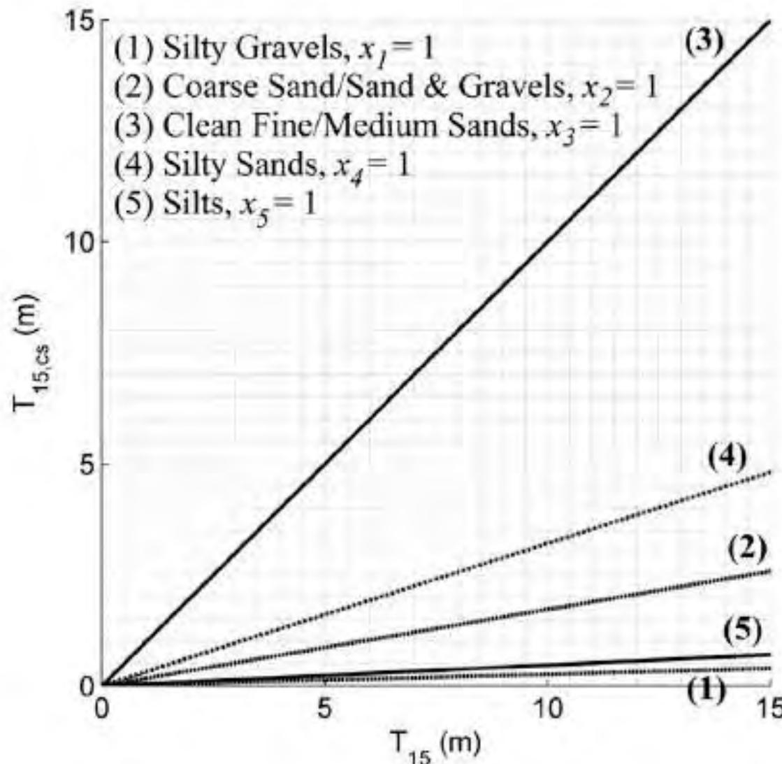
Fig. 3.  $T_{15}$  versus  $T_{15,cs}$  according to soil index
