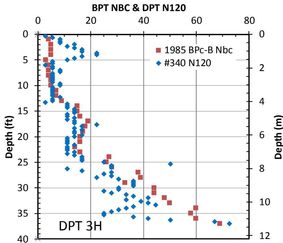
$$N_{120} = N_{\text{measured}} \left( E_{\text{Delivered}} / E_{\text{Chinese DPT}} \right)$$
