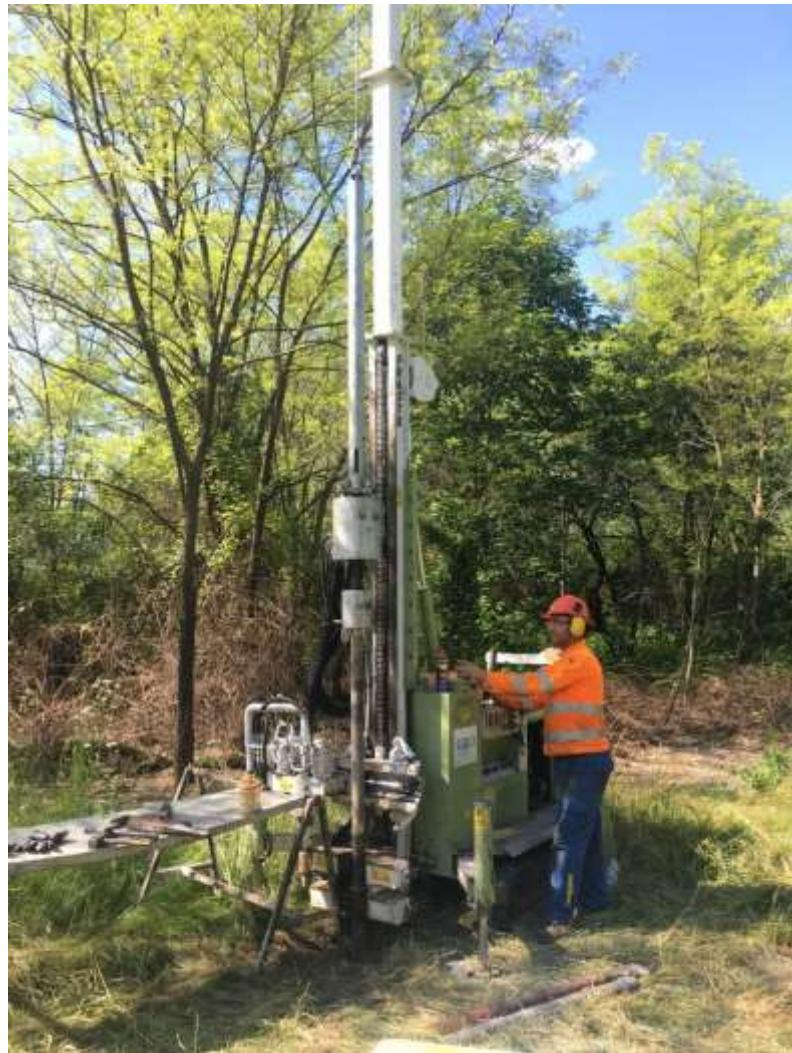
Testing with 154 kg Hammer-0.67 m drop
