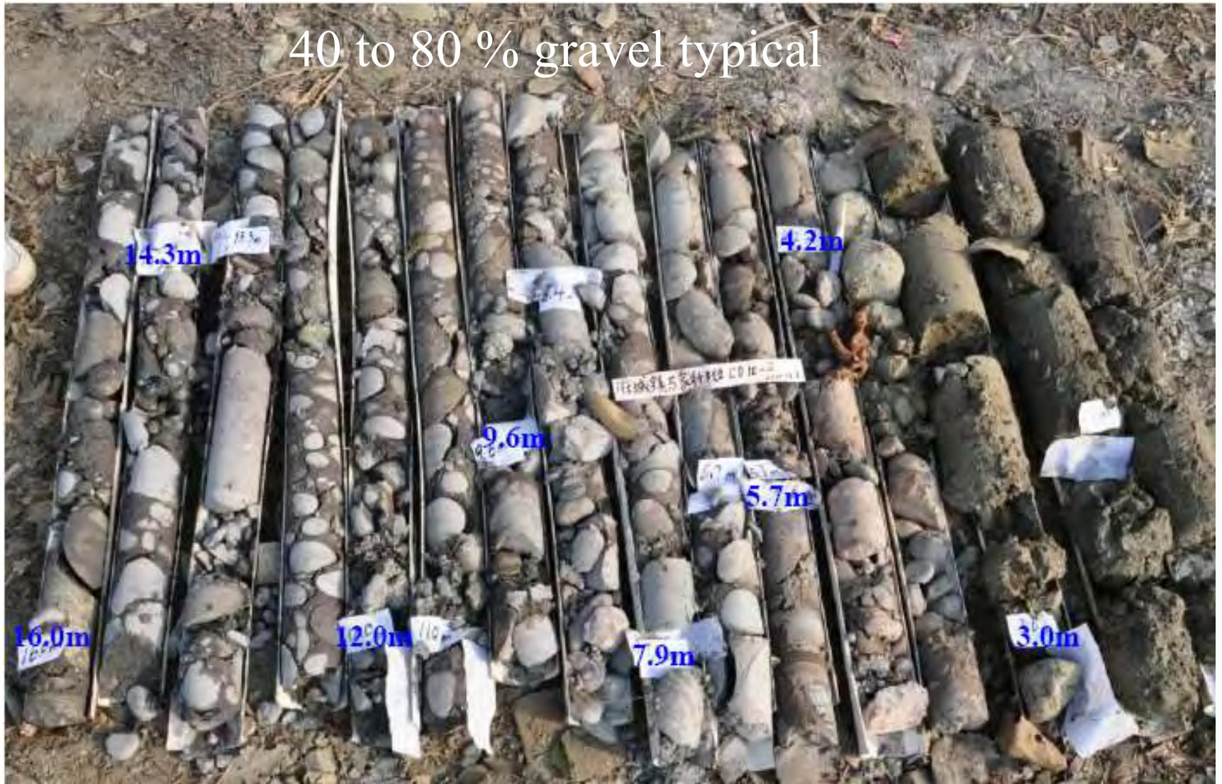
Core samples from borehole near a DPT sounding showing gravelly and cobbly composition of sediment penetrated beneath Chengdu Plain
