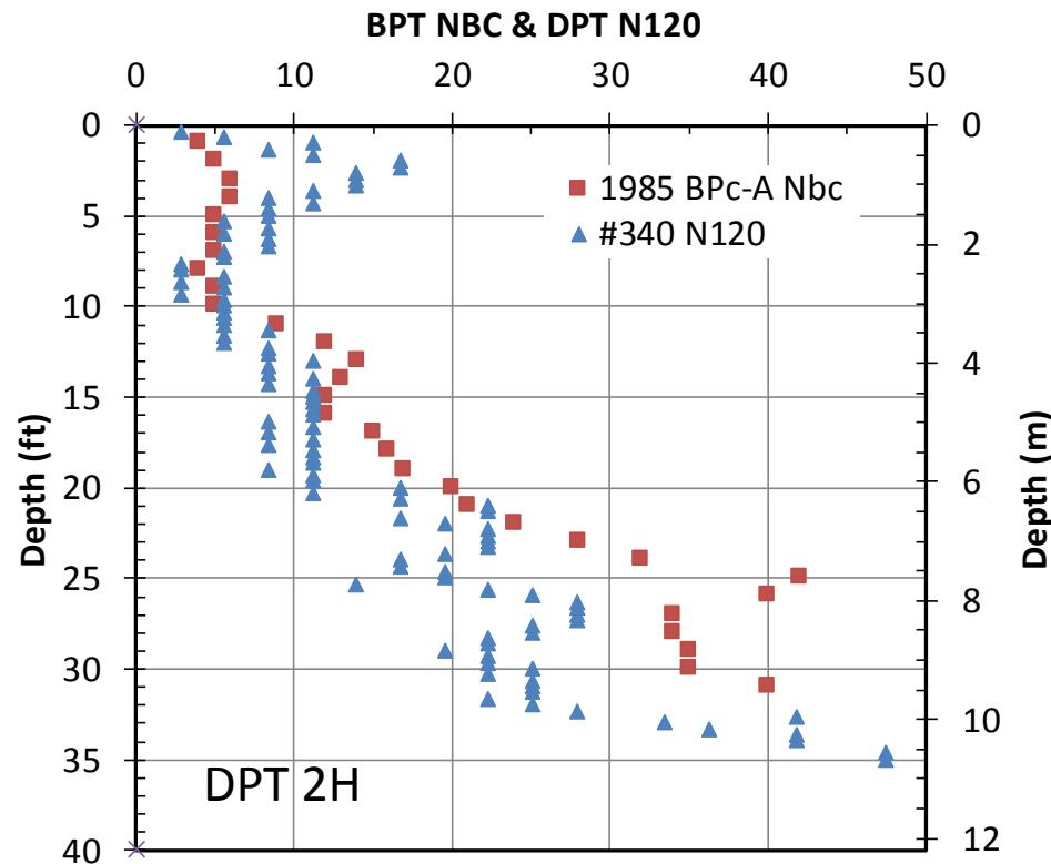
$$N_{120} = N_{\text{measured}} \left( E_{\text{Delivered}} / E_{\text{Chinese DPT}} \right)$$
