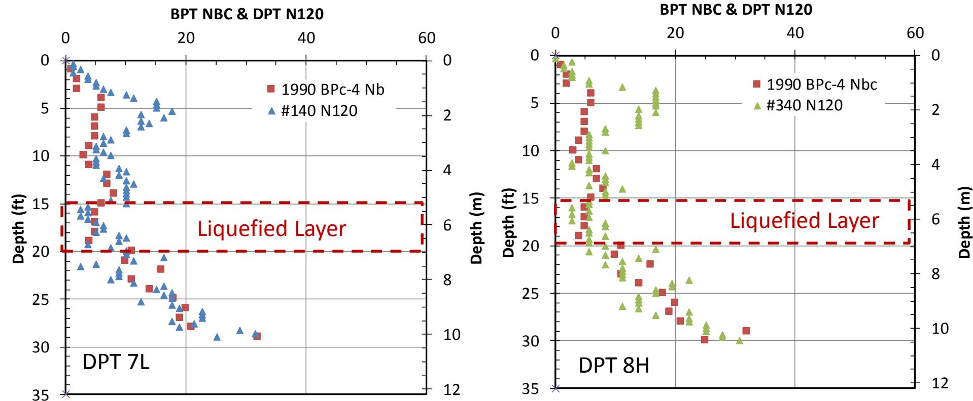
$$N_{120} = N_{\text{measured}} \left( E_{\text{Delivered}} / E_{\text{Chinese DPT}} \right)$$
