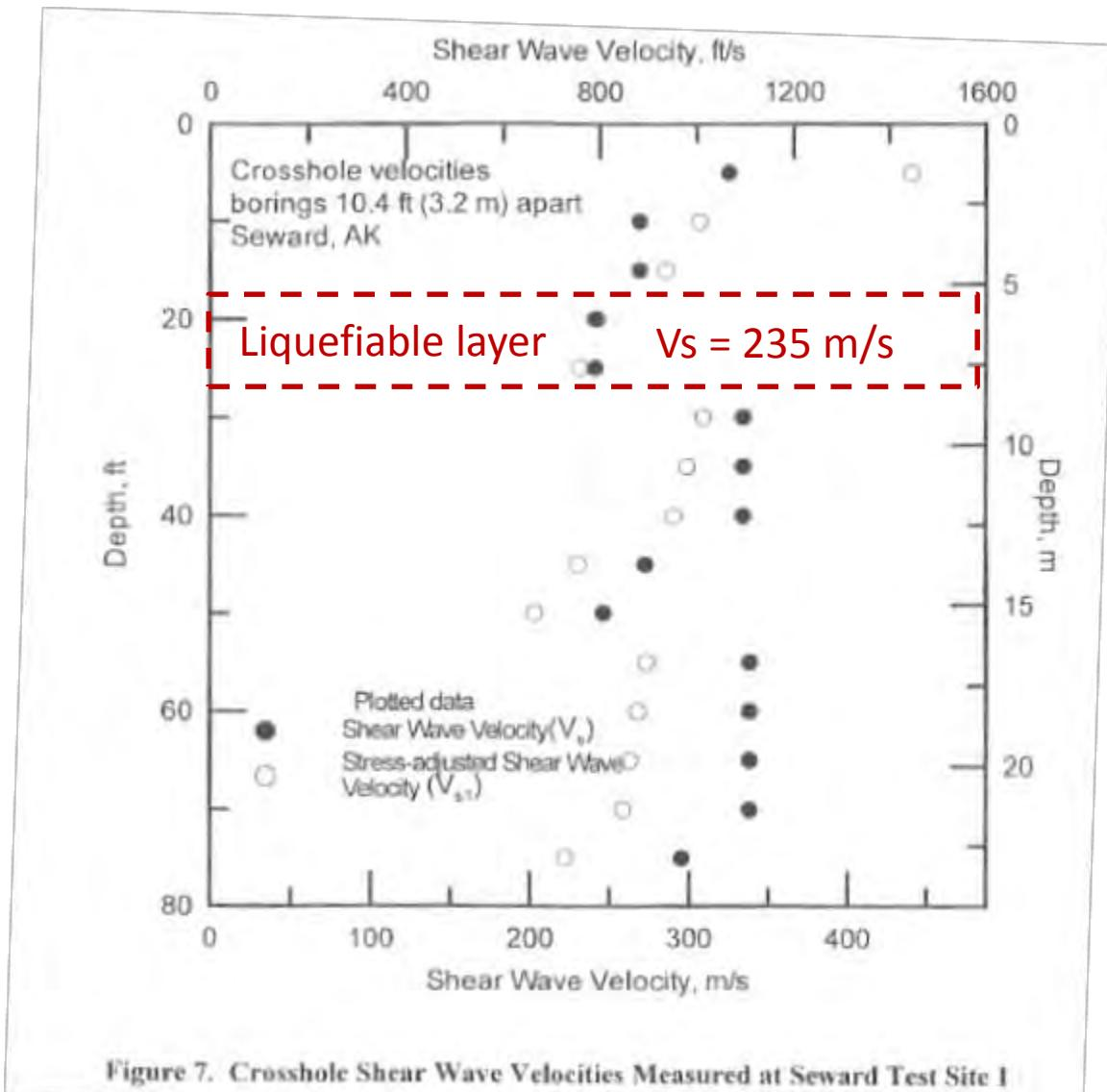
Figure 7. Crosshole Shear Wave Velocities Measured at Seward Test Site 1
