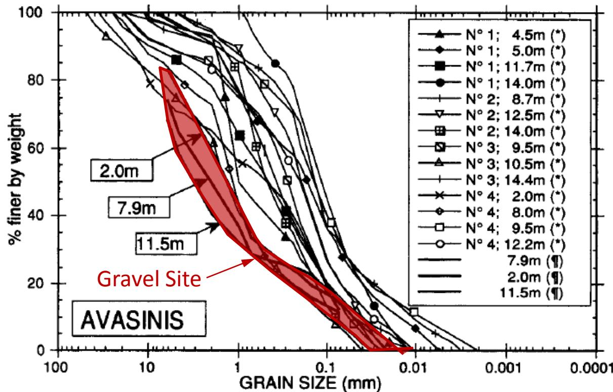
**Fig. 5.** Grain size distributions of Avasinik sediments: (\*): four sites from F. Sgobino (private communication), liquefied or suspected of liquefaction. (¶): from the site investigated in the present study, extensive liquefaction
